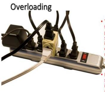
The most common cause of fires from extension cords, power strips, power taps, or surge protectors is due to improper use and overloading, especially when cords have multiple outlets such as power strips and/or surge protectors.
